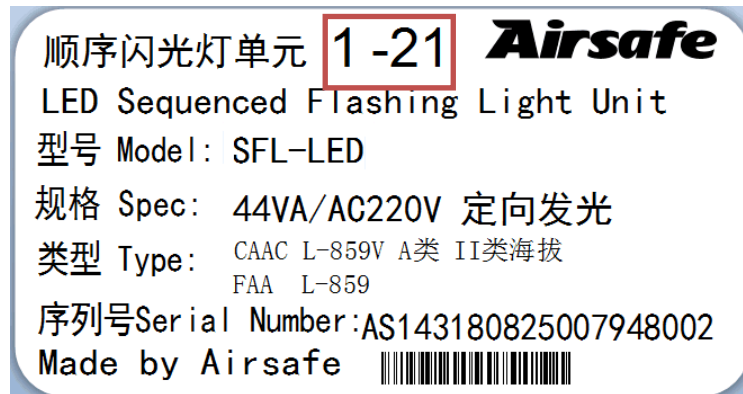
Figure3.1 Label of lighting fixtures
