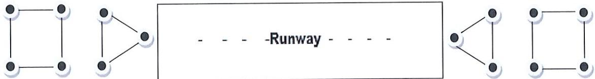
Positioning of foundation bolt for triangular and square masts, in relation to the runway.
