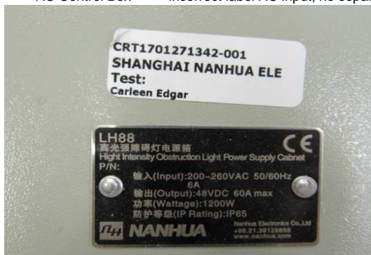
AC Control Box * incorrect label AC input, no separate part number
