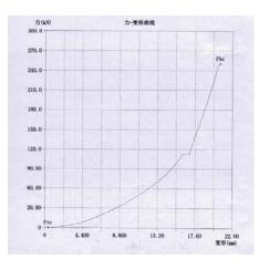
Note: pressure test with the rubber pad
